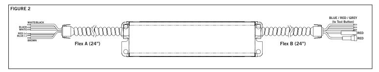
Complete wiring as indicated below. Install in accordance with National Electric Code. Emergency Pack and AC Driver must be on the same branch circuit. Ensure hot / live lead going to the black wire on the Emergency LED driver is Un-Switched. When used with switched fixtures, the emergency pack must be wired ahead of the switch. (See Figure 3.)
