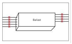
From mains, connect input (L) line to all wires coming from sockets on one side of sign and (N) neutral to all wires coming from the sockets on opposite end of the sign.
