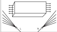
Insert Keystone Sign Hero LED tubes and rotate to desired position for optimal illumination. Ensure side marked "L" is connected to corresponding line socket and "N" is connected to corresponding neutral socket.
