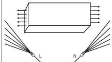
Insert Keystone Sign Hero LED tubes and rotate to desired position for optimal illumination. Ensure side marked "L" is connected to corresponding line socket and "N" is connected to corresponding neutral socket.
