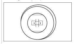
Access sign raceway/wiring box, and cut all ballast input and output wires as shown. Do not remove ballast if removal leaves an opening in the raceway.
