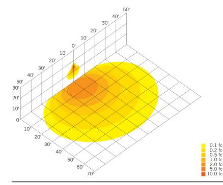
Ground mounted at 6" above ground, 10° above horizontal, shining towards building exte-
