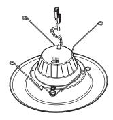
**6.** Plug E26 base cable connection into the recessed housing.
