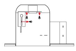
**3.** Remove existing socket mounting plate from the housing, then remove lamp socket from the plate.
