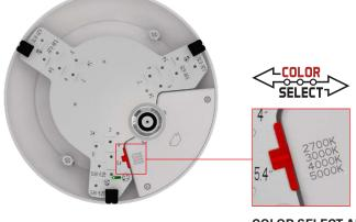
**COLOR SELECT ADJUSTMENT SWITCH** Set dip switch to adjust CCT between 2700K, 3000K, 4000K, and 5000K. Fixture comes preset at 2700K.
