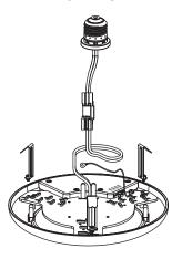
7. Secure fixture ground (green) wire to the recessed housing.
