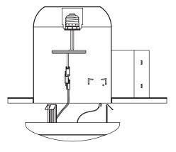
**9.** Push the disk light up until light is flush with ceiling.
