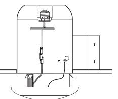
8. Guide the disk light into the housing for a tight fit.
