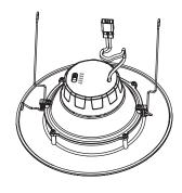
**6.** Plug E26 base cable connection into the recessed housing, ensuring that kit is grounded.
