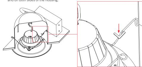
**8.** Carefully place wires into housing, then push the LED trim into the housing until trim is flush with ceiling.
