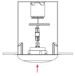
**9.** Push the disk light up until light is flush with ceiling.
