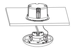
4. Carefully tuck wires inside J-Box, align springs with bracket center and push disk light up inside J-Box until flush with the ceiling surface.
