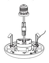
**6.** Screw E26 base adaptor into the recessed housing.
