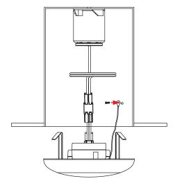
**8.** Guide the disk light into the housing for a tight fit.
