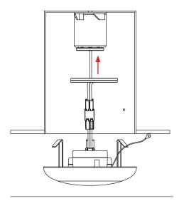
**7.** Secure fixture ground (green) wire to the recessed housing.
