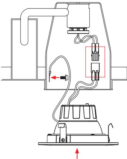
5. Carefully route wires into fixture, sliding the trim and friction clips into the housing for a tight fit.
