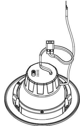
4. Plug E26 base cable connection into the recessed housing kit, ensuring that kit is grounded.
