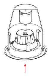
**6.** Push the LED trim into the housing until trim is flush with ceiling.
