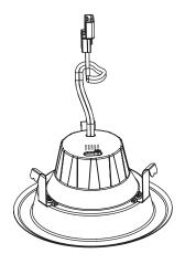
**4.** Plug E26 base cable connection into the recessed housing.
