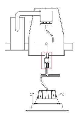
Carefully route wires into fixture, sliding the trim and friction clips into the housing.
