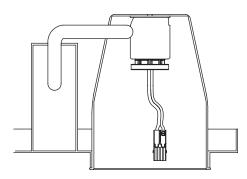
Select desired CCT using adjustment switch on driver box (see Color Select (CCT) Adjustment on page 3).
