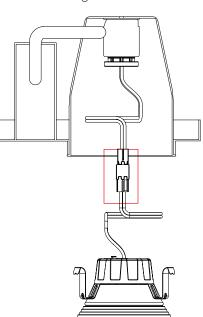
**5.** Carefully route wires into fixture, sliding the trim and friction clips into the housing.
