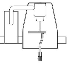
**3.** Select desired CCT using adjustment switch on driver box (see *Color Select* (*CCT*) *Adjustment* on page 3).
