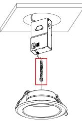
8. Lifting both retention tabs upward, push the fixture into the hole until trim sits flush with ceiling.
