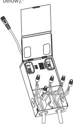
Place all wiring and connections back into the box and close the cover.
