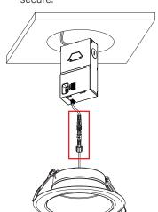
**8.** Lifting both retention tabs upward, push the fixture into the hole until trim sits flush with ceiling.
