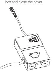
7. Insert driver box into ceiling in accordance with local/national codes and connect the male and female connectors. Screw threaded nut over connectors to secure.
