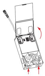
5. Insert the electrical supply cable through the KO; use appropriate bushing to prevent wire abrasion. Wire driver box (see *Wiring Diagram* on page 3 and illustration below).\*
