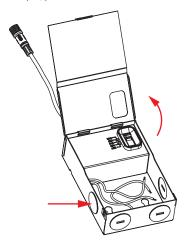
5. Insert the electrical supply cable through the KO; use appropriate bushing to prevent wire abrasion. Wire driver box (see *Wiring Diagram* on page 3 and illustration below).\*
