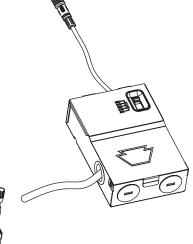
7. Insert driver box into ceiling in accordance with local/ national codes and connect the male and female connectors. Screw threaded nut over connectors to secure.
