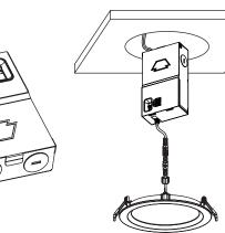
**8.** Lifting both retention tabs upward, push the fixture into the hole until trim sits flush with ceiling.
