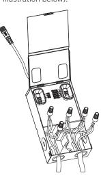
8. Lifting both retention tabs upward, push the fixture into the hole until trim sits flush with ceiling.
