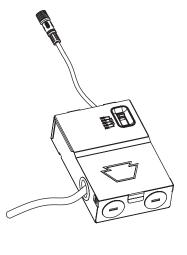
7. Insert driver box into ceiling in accordance with local/national codes and connect the male and female connectors. Screw threaded nut over connectors to secure.
