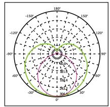
Maximum Candela = 1248.55 Located at Horizontal Angle = 0, Vertical Angle 0
