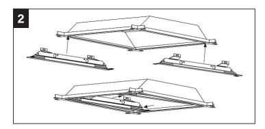
3. Insert the two side bars into the clearance between the brackets and the T-grid.
