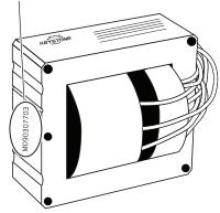
Ten Digit Date Code (Ballast with "VersionP\_" indicated on the unit label) Example: M090307703
