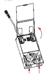
5. Insert the electrical supply cable through the KO; use appropriate bushing to prevent wire abrasion. Wire driver box (see *Wiring Diagram* on page 3 and illustration below).\*
