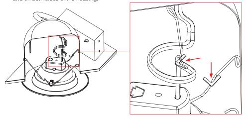
**6.** Carefully place wires into fixture, then push the LED trim into the housing until trim is flush with ceiling.
